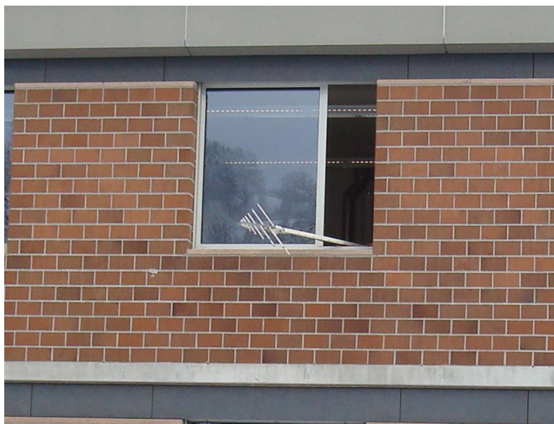
Figure 8: Stability measurements are performed with an antenna placed at a fixed position in front of the opened window.
