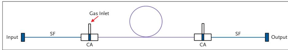
2: Schematised all-fibre cell; HCF: hollow-core fibre; SF: standard silica fibre; CA: connector adapter.
