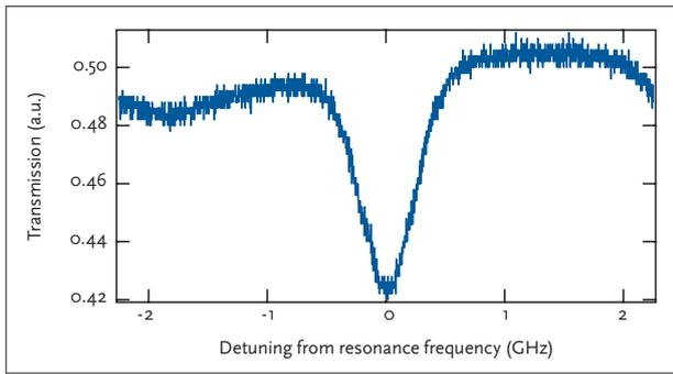
7: P16 line of  $^{13}\text{C}_2\text{H}_2$  as seen by tuning an AFTL source around the resonance frequency.
