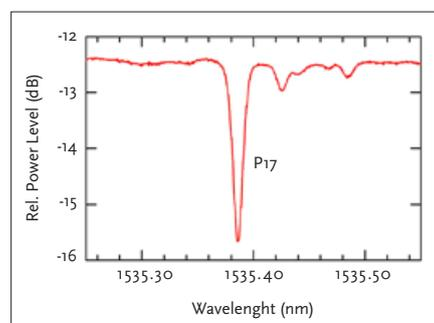
6: Doppler linear absorption of the P17 line of  $^{12}\text{C}_2\text{H}_2$ .
