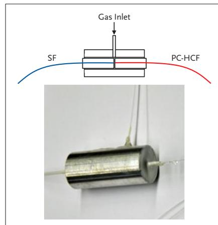
4: Gas tight connector adapter, principle and practical realisation.
