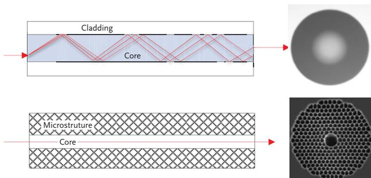
1: Two different guiding mechanisms: Total reflection in standard fibres (top), and photonic bandgaps (bottom).
