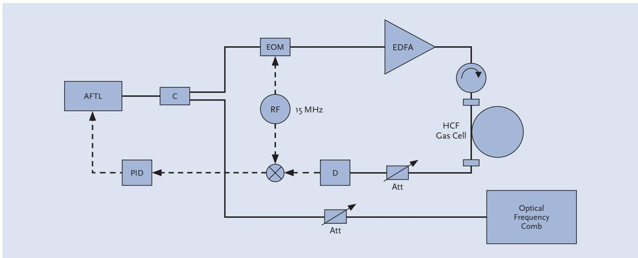
9: All-fiber optical setup for linear spectroscopy and laser stabilisation. AFTL: all-fiber tuneable laser; C: coupler; EOM: electro-optic modulator; EDFA: erbium-doped fiber amplifier; Att: attenuator; D: detector; PID: proportional-integral-derivative controller for laser lock. The Optical Frequency Comb allows to measure the frequency stability of the stabilised laser.
